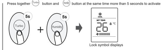
At lock mode, all buttons will not response except pressing these two buttons for two seconds again to disable locking.
