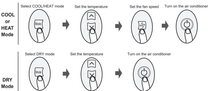
In DRY mode, fan speed can not be set since it has already been automatically controlled.
